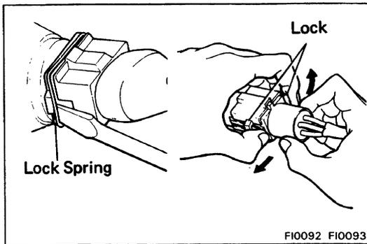
8. Care is required when pulling out and inserting wiring connectors.
