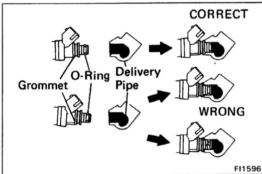
3. Observe the following precautions when removing and installing the injectors.
