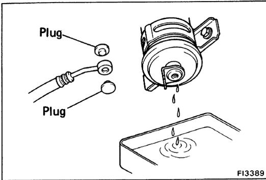
1. When disconnecting the high fuel pressure line, a large amount of gasoline will spill out, so observe the following procedure:
