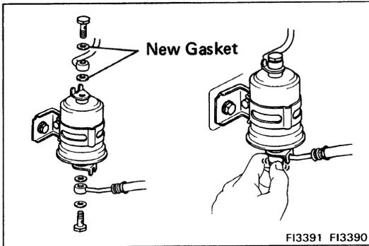
2. When connecting the flare nut or union bolt on the high pressure pipe union, observe the following procedure: (Union Bolt Type)
