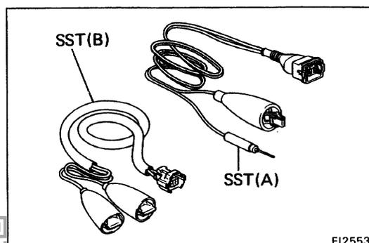
10. Use SST for inspection or testing of the injector, cold start injector or its wiring connector.
